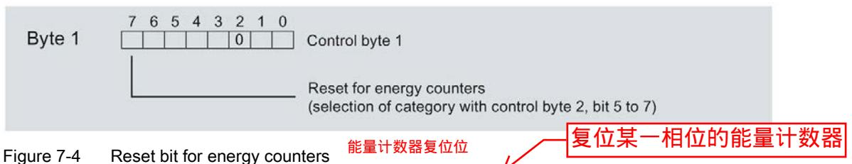
Figure 7-4 Reset bit for energy counters
