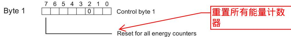
Figure 7-5 Resetting the energy counters for module version with 2 bytes of output data
